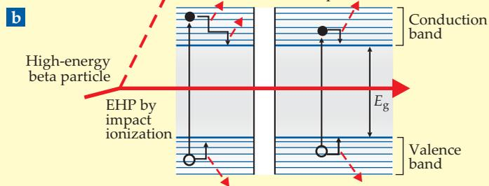
sorbed in less than a micron of Sc or Ti. But that problem can largely be solved by stacking thin alternating layers of metal tritide and semiconductor in the desired geometry. That approach allows for a higher energy density for a tritium betavoltaic without the concerns associated with gaseous tritium, especially at high pressures. Assuming a
