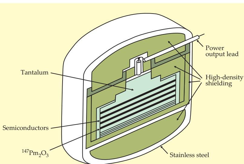
**Figure 1. The Betacel model 400**, an early betavoltaic battery powered by promethium-147. The device was produced for use in cardiac pacemakers.
