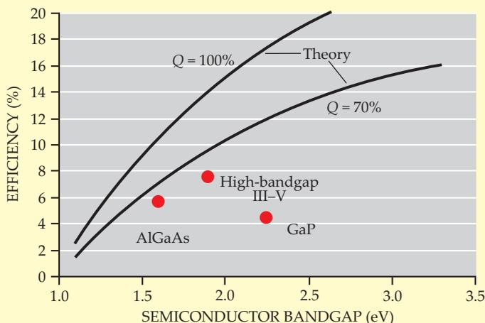
**Figure 3. Some recent efficiency measurements** for tritium betavoltaics using aluminum gallium arsenide,<sup>5</sup> gallium phosphide,<sup>7</sup> and a high-bandgap III–V semiconductor,<sup>11</sup> compared with the theoretical maximum efficiency as a function of bandgap. Theoretical curves are shown for collection efficiencies  $Q$  (the current generated relative to the maximum possible current) of 100% and 70%.
