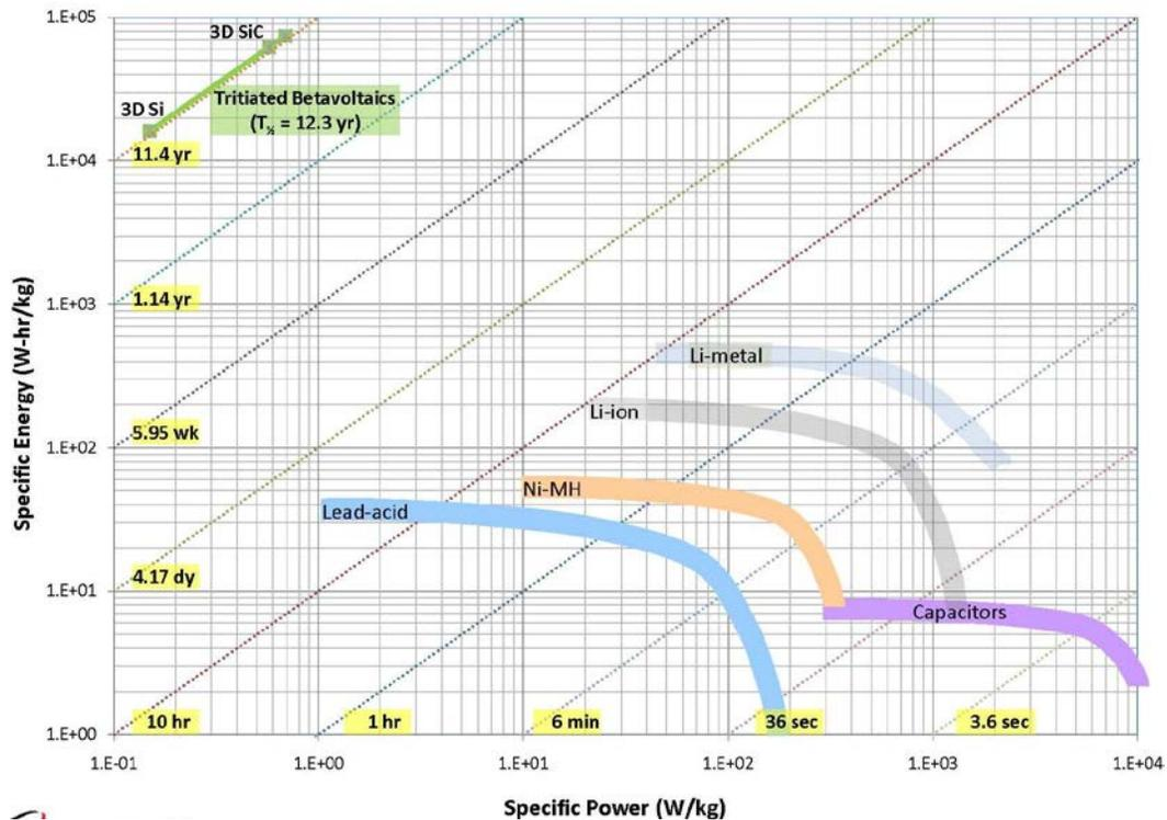
Figure 2. Ragone Plot for Batteries and Betavoltaics. The diagonals labeled with time give an indication of the power delivery period for the technologies shown. (Battery & Capacitor Data: <http://berc.lbl.gov/venkat/Ragone-construction.pps>)
