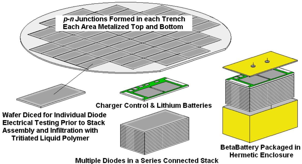
Figure 1. Prototype BetaBattery™ fabrication and assembly steps.
